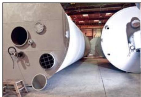
*Two of the Portasilo steel storage vessels under construction, showing (right) internal welding inspection.*
